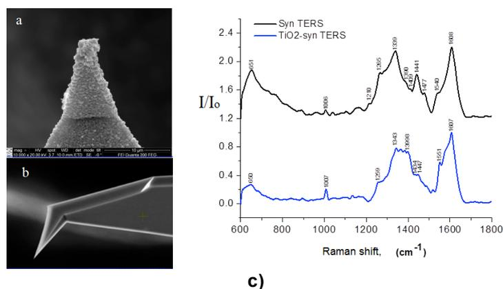
**Figure 1.** AFM-TERS probes used in experiment: a) silver chemically decorated apex of the probe, b) NT-MDT probe based on so-called “Top Visual” AFM Si cantilevers. TERS spectra of  $\alpha$ -synuclein ( c).
